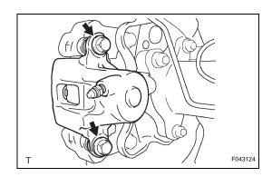
(b) Install the disc brake cylinder onto the disc brake cylinder mounting with the 2 slide pins.
